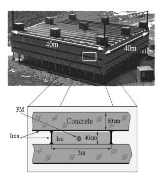
Figure 1. The ANI calorimeter structure, with an expanded drawing of one cell of the ice Cherenkov detector, as discussed in the text.
